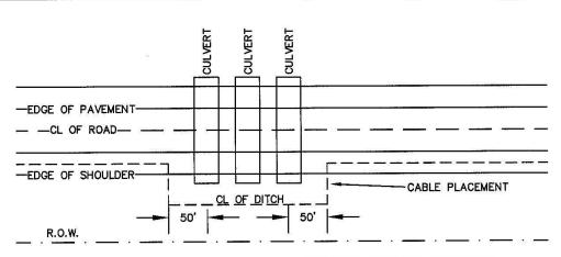
TYPICAL DETAIL OF THE PLACEMENT OF CABLE AROUND CULVERTS
