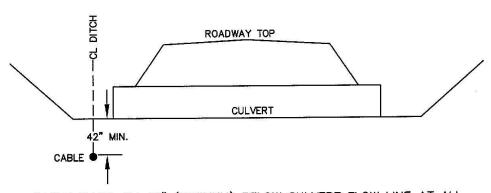
CABLE SHALL BE 42" (MINIMUM) BELOW CULVERT FLOW LINE AT ALL CULVERTS WHERE CABLE IS PLACED AROUND THE END OF CULVERT. NOT TO SCALE
